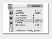
CH 4 CHANNEL To store the fine tuning Antenna ANT/CATV **4** A ▶ **4** ANT ▶ setting in the TV's memo-ANT/CATV Auto Program Fav. Channel Fine Tune Labeling Blue Screen ry, move the joystick up. 韗 **4** +03 ♥ ▶ (A heart icon will appear.) To reset the fine tuning to "00," move the joystick down. Press the Menu button to exit.
